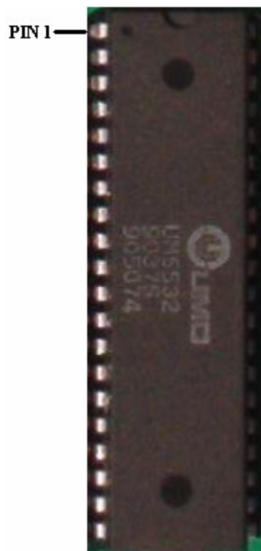
Figure 5: IC showing pin 1
